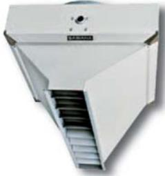
The ATLAS Sabiana STP Door Curtain unit with its special fishtail diffuser is designed to provide a screen of warm air across the door opening to restrict cold air blowing into the area and to reduce the heated atmosphere inside the area from escaping out.
